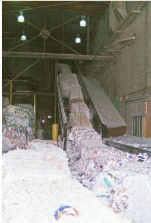
Recycled fiber moving up the conveyor; a scanner at the top reads the RFID tags
